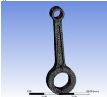
Fig. 2 Meshing of Two wheeler connecting rod
